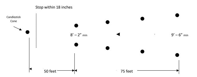
\* Measure distance between cones from the base of the cones
