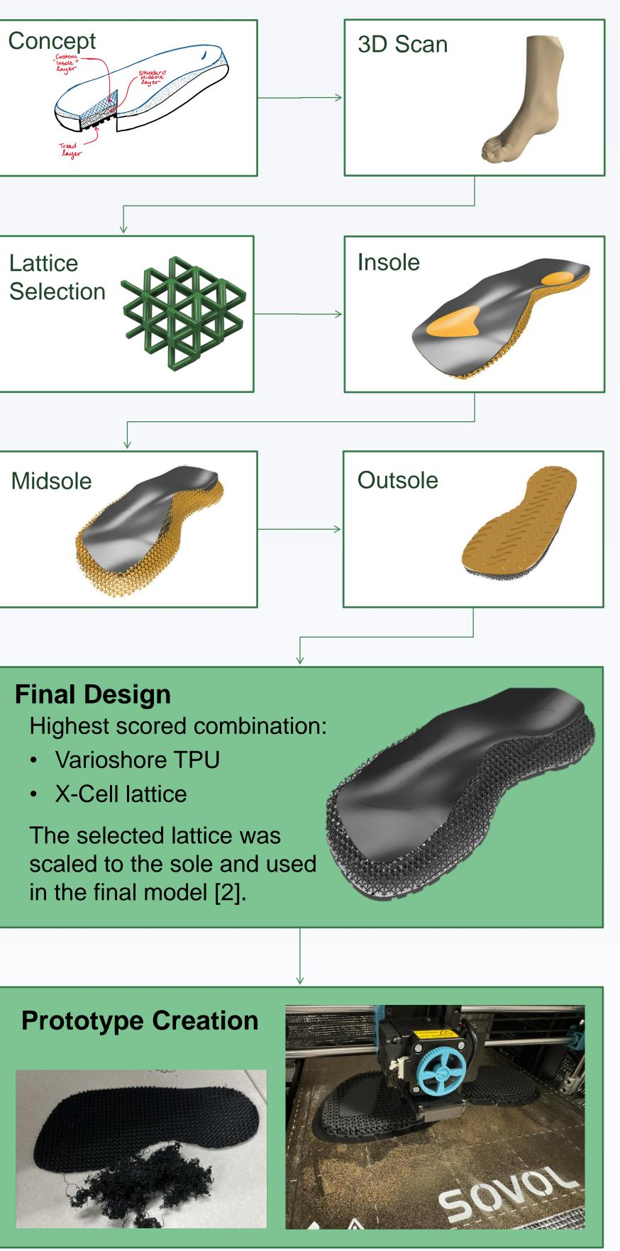
A sole was designed and successfully constructed using an additive manufacturing process. The results were incorporated into a fully functional midsole by narrowing the scope of the project using customer feedback. Using a 3D scan of any foot, the model can easily be customized to any individual user. Further research could explore additional factors such as environmental sustainability, manufacturing feasibility, and user preferences to refine and optimize sole design.
