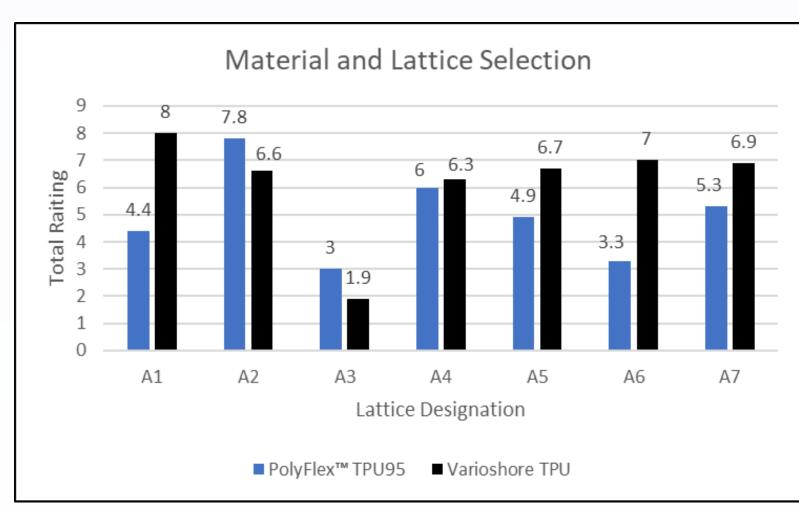
Samples were ranked based on performance from each test and total cost to produce. An x-cell structure with Varioshore TPU had the highest cumulative rank.
