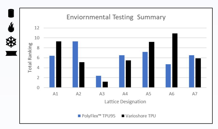
Samples were put through environmental testing and compared with original samples. Samples A3 of both materials fractured.
