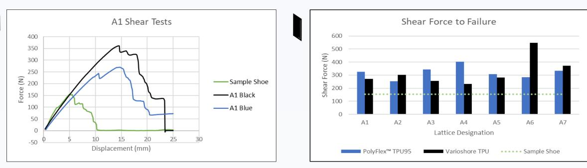
All samples outperformed the sample shoe at resisting shear.
