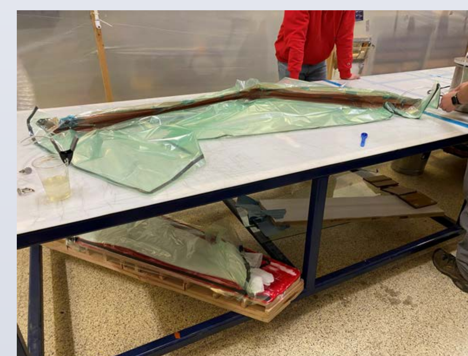
Figures 4 & 5: Applying carbon fiber layers and vacuum sealing connection rod.
