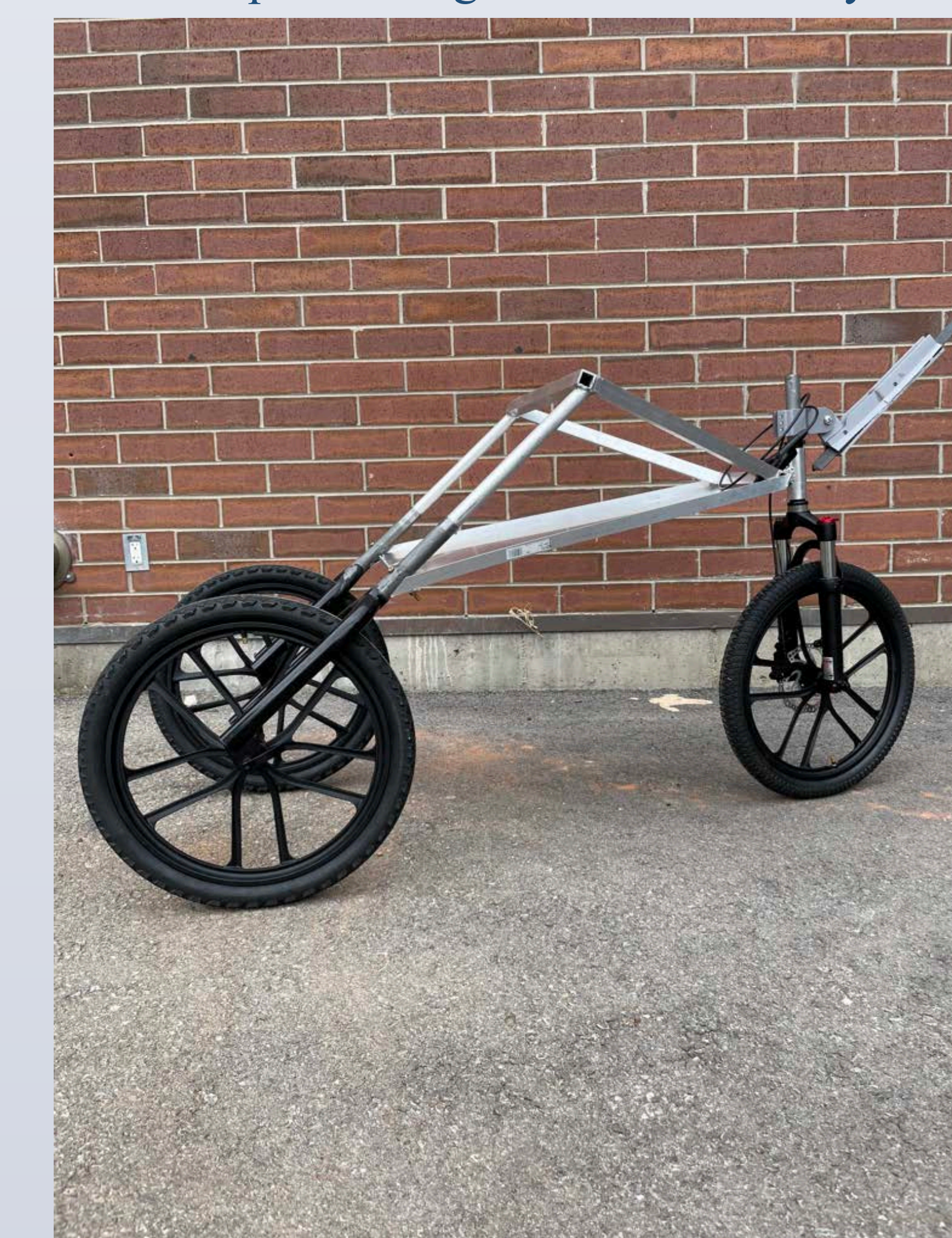
Figure 8: Nearly completed assembly of the frame of the cart.
