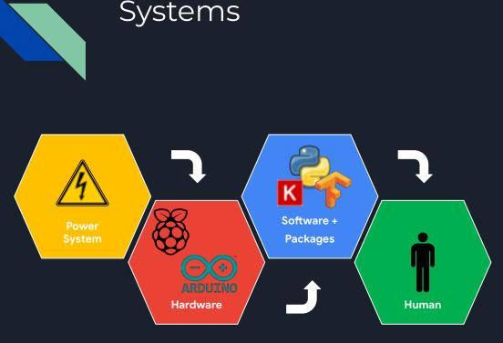
The system that sorts the fish is based on the concept of deep learning image recognition. The primary computing device that compares the fish to the trained image model is a single board raspberry pi 4 computer. This is the primary decision maker in the sorting process.
