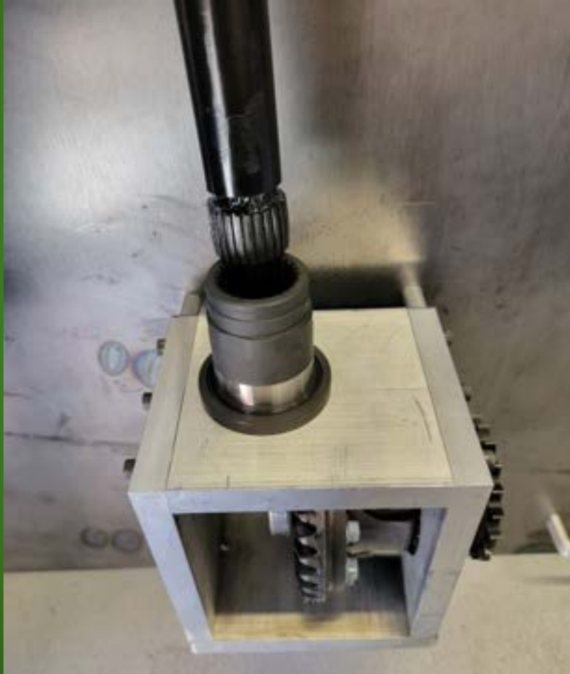
Drive Shaft - Rear Gear Box
