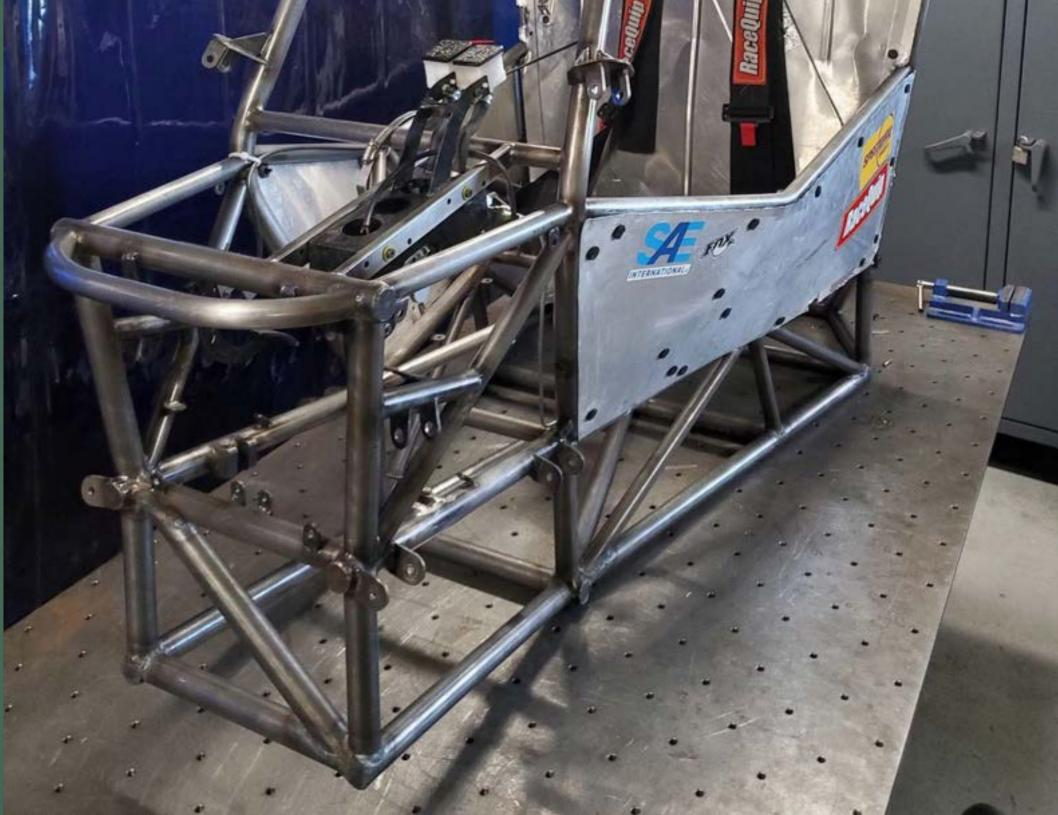
Assembled subframe showing overall addition to vehicle frame. Suspension mounting points will be translated down onto the subframe.
