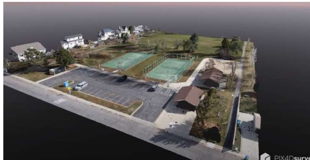
Figure 3. 3D model created using drone photogrammetry.
